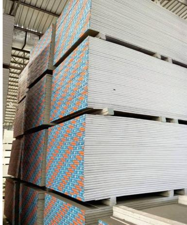
2. **Green Board** - Moisture resistant type that is used in high humidity areas (Wet areas) for both ceiling & partition.
